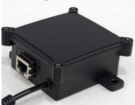
Figure 2. "CARKIT" Radar sensor demonstrator in the housing 50x50x30mm
